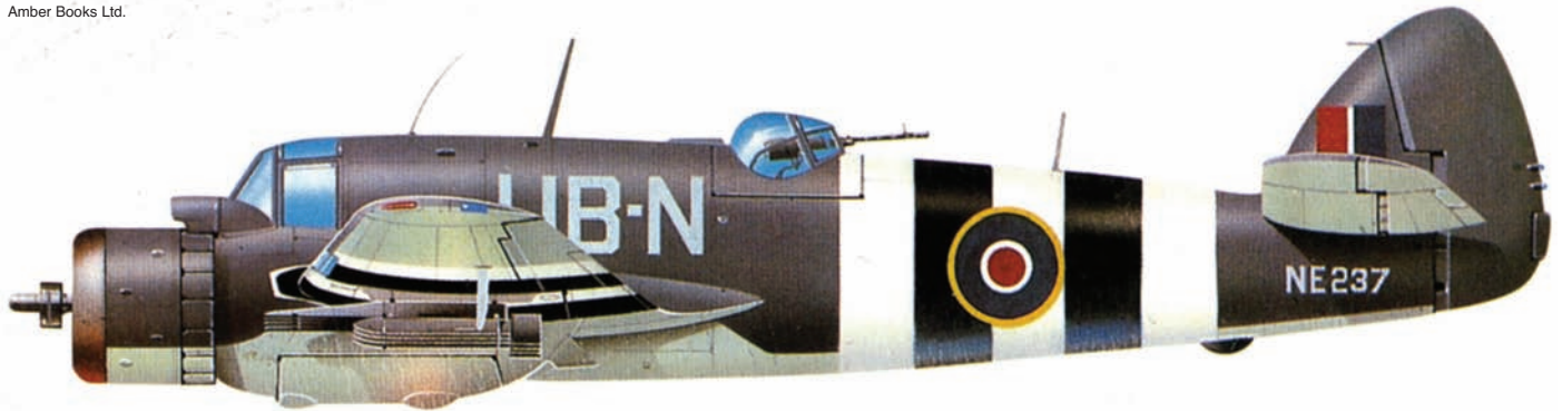
This drawing of a Bristol Beaufighter TF Mk X of No. 455 Squadron, Royal Australian Air Force, presents the aircraft's distinctive profile with its large hump and dorsal machine-gun position.
