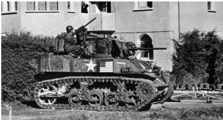
ABOVE: This Stuart light tank is equipped with a 37mm main weapon and a .30-caliber machine gun in the turret glacis for defense against enemy infantry. This photograph was taken in the city of Casablanca a few days after the Operation Torch landings. BELOW: In this area south of Mehdia Plage, a pivotal tank battle took place between American and Vichy French armored forces. In the distance beyond the lake lies the Kasbah, where a garrison of 250 Vichy French troops had to be neutralized.
