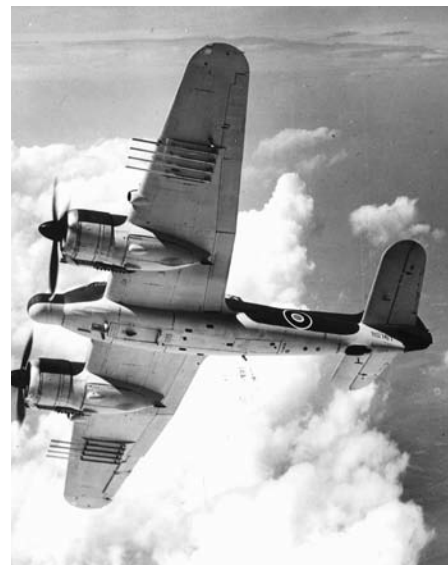
ABOVE: The dependable Beaufighter was one of the earliest aircraft to perform in multiple roles during World War II. LEFT: This Bristol 156 Beaufighter TF Mk X, operated by Royal Air Force Coastal Command, is outfitted with torpedoes and rockets for use against enemy shipping.
