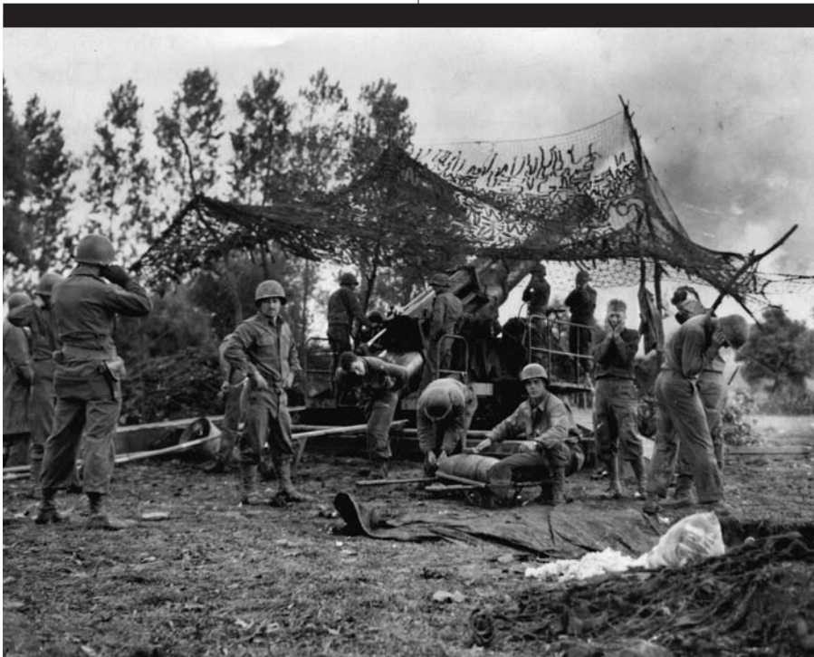
ABOVE: A super-heavy 240mm M1 howitzer blasts German positions to break up an enemy tank attack. Maximum range was over 25,000 yards. OPPOSITE: Shermans line up in an unidentified French city, September 27, 1944, in preparation for a continuation of the drive toward the German border.
