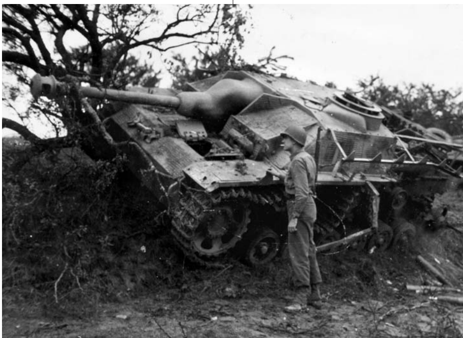
A GI examines a knocked-out StuG IV near Lunéville, France. The StuG IV had no rotatable turret; the entire vehicle had to be aimed in the direction of the target.
