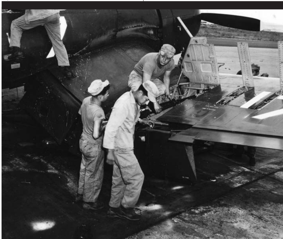
ABOVE: Ground crewmen install one of the Corsair's six .50-caliber machine guns. BELOW: Marine mechanics at an air field work on a jeep engine.
