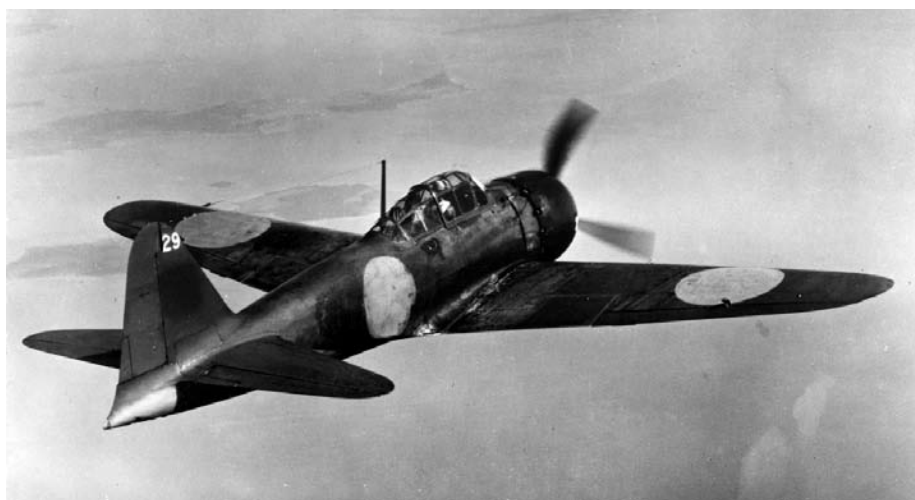
TOP: The U.S. Navy F6F Hellcat showed superior performance to the Japanese Zero in air speed and when climbing and diving. ABOVE: The Japanese A6M Zero's fuselage and wings were constructed in one piece that made the aircraft sturdy and highly maneuverable. RIGHT: U.S. Admiral Raymond Spruance (left) and Japanese Vice Adm. Jisaburo Ozawa.
