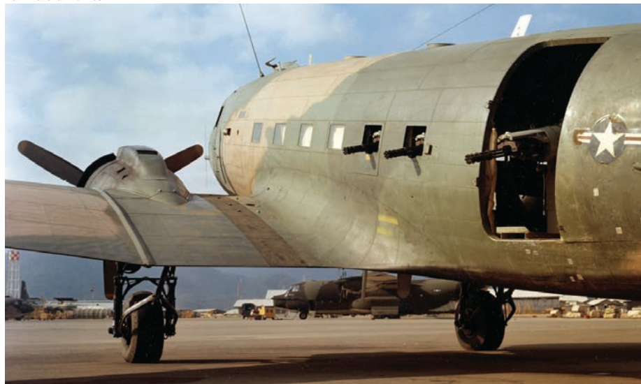
ABOVE: An AC-47D at Nha Trang Air Base displays the three 7.62mm miniguns that make up its armament. The miniguns were positioned on the left side of the aircraft so that it could furnish continuous fire while circling. BELOW: An AC-47D crew test fires a 7.62 minigun in November 1966.
