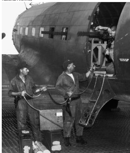
The crew of an AC-47 loads 7.62mm miniguns that can fire up to 18,000 rounds per minute. Beside them on the ground are boxes of ammunition and flares.
