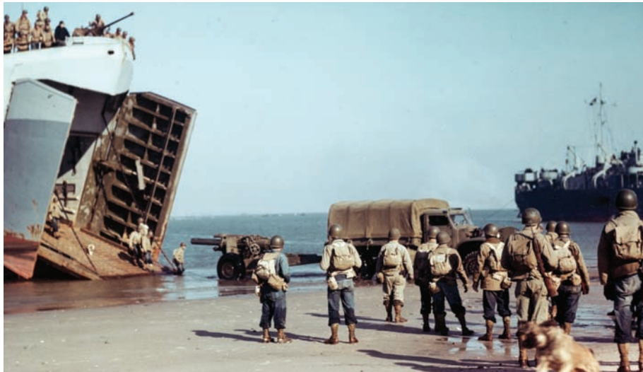
ABOVE: LSTs (landing ship, tank) were the backbone of amphibious cargo and personnel transport on a tactical level. In this photo taken at the Amphibious Training Base at Camp Bradford, Virginia, sometime in 1943-1944, an LST offloads an Army truck with a towed howitzer. OPPOSITE: Photographed with an LCT (landing craft, tank) lashed to its deck, LST 940 rides at anchor. On May 14, during rehearsal for the Saipan invasion, three LCTs broke loose from their LSTs and two sank in the ocean during a storm. Unfortunately, a number of Marines sleeping in the LCTs were missing or killed when the LCTs pitched off the LSTs.
