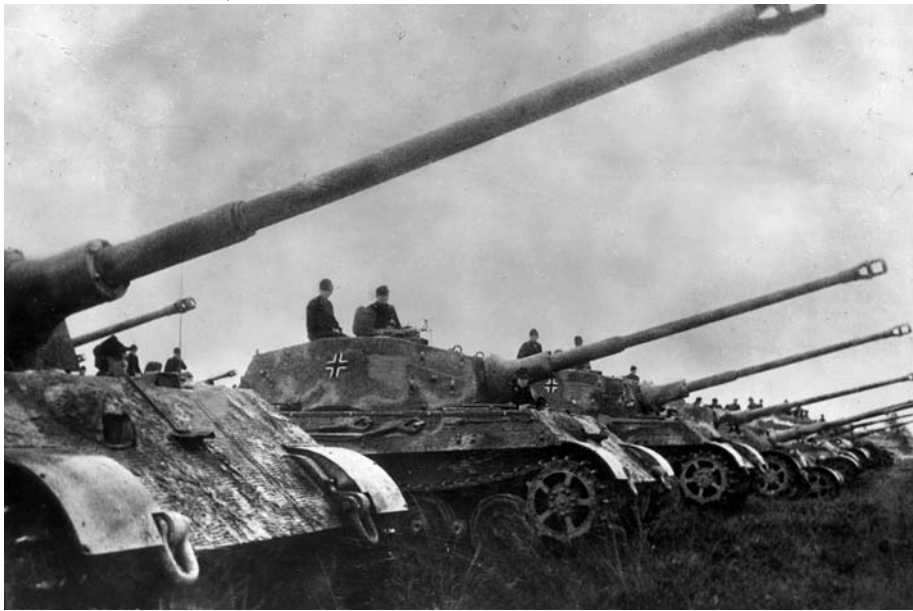
The German Tiger II tank with a deadly 88 PaK 43 cannon could carry on board 40 HE and 40 AP rounds.
