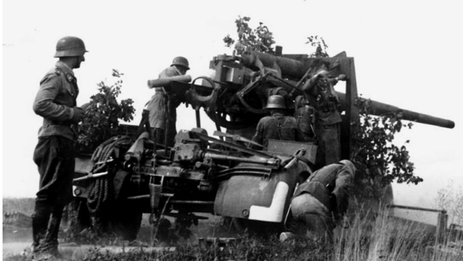
An 88mm gun on the Eastern Front in 1941. A 1944 German ordnance listing included 19 different types of rounds: eight high explosive (HE), seven armor piercing (AP), and four kinetic energy.
