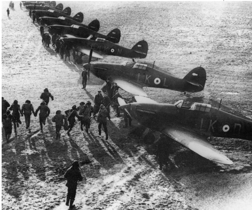
ABOVE: RAF pilots scramble to their Hawker Hurricane fighters to defend the skies over England. Much of the Hurricane was covered with fabric, rather than metal, making it easier to build and easier for ground crews to repair. LEFT: Luftwaffe Commander-in-Chief Hermann Göring inspects captured Allied aircraft. He unrealistically promised Adolf Hitler that he would defeat the Royal Air Force in time for Operation Sea Lion, the amphibious invasion of England.
