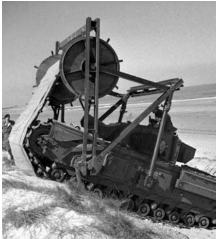
The Churchill ARVE Bobbin featured a 10-foot-wide canvas cloth reinforced with steel poles that unrolled onto the ground. The canvas offered traction over the soft sand of the invasion beaches.
