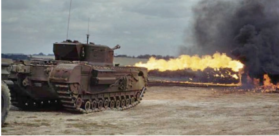
ABOVE: The Crocodile's flamethrower was connected to an armored trailer that carried 400 gallons of flammable fuel. BELOW: Most of the retrofitting involved modifications to the British Churchill tank or to the U.S. Sherman tank. The Sherman amphibious tank outfitted with a watertight canvas housing was designed to float to shore from a landing craft at sea. Heavy seas on D-Day caused a number of these tanks to sink, drowning their crews.
