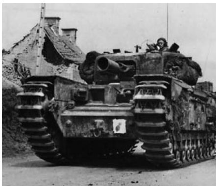
ABOVE: The Sherman Crab featured a rotating cylinder with weighted chains designed to detonate mines for follow-on forces. BELOW: The Churchill AVRE Fury featured a petard mortar that fired a 40-pound projectile intended for use against concrete bunkers and roadblocks.
