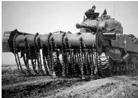
ABOVE: The Sherman Crab featured a rotating cylinder with weighted chains designed to detonate mines for follow-on forces. BELOW: The Churchill AVRE Fury featured a petard mortar that fired a 40-pound projectile intended for use against concrete bunkers and roadblocks.
