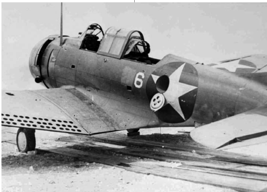
This Douglas SBD-2 Dauntless dive bomber, flown by Lieutenant Daniel Iverson with his gunner Private Wallace Reid, was one of only eight from VMSB-241 to return from the attack against the Japanese fleet on June 4. The plane had 219 holes from enemy fire.
