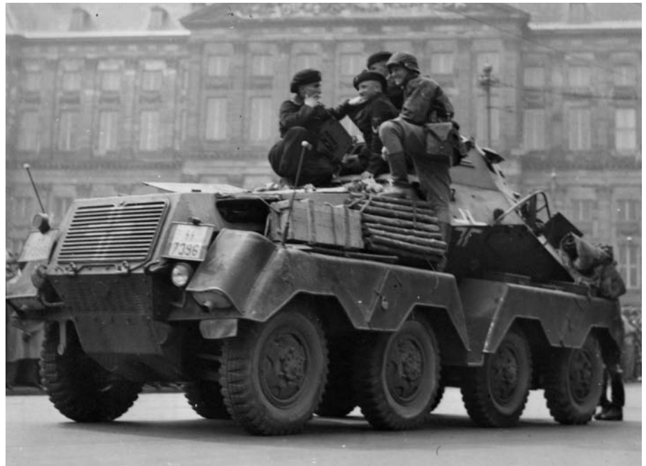
Scout troops clad in panzer uniforms and berets sit atop an Sdkfz.231 (8-rad) heavy armored reconnaissance vehicle.
