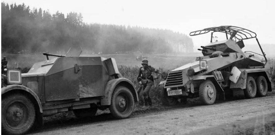
Reconnaissance troops participate in an exercise in 1936 with an Sdkfz.13 open-topped armored scout car armed with an MG-13 machine gun and a Sdkfz.232 six-wheeled heavy armored scout vehicle featuring a fully rotating turret with a 20mm autocannon and an MG-13 machine gun.
