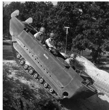
ABOVE: An M-29C Weasel demonstrates its ability to traverse difficult terrain during maneuvers. The tracked Weasel proved to be a versatile performer. TOP: This M-29 Weasel amphibious tracked vehicle of Company C, 1st Engineer Combat Battalion, 29th Infantry Division has been nicknamed the St. Lo Special . This photo was taken in France during the summer of 1944.
