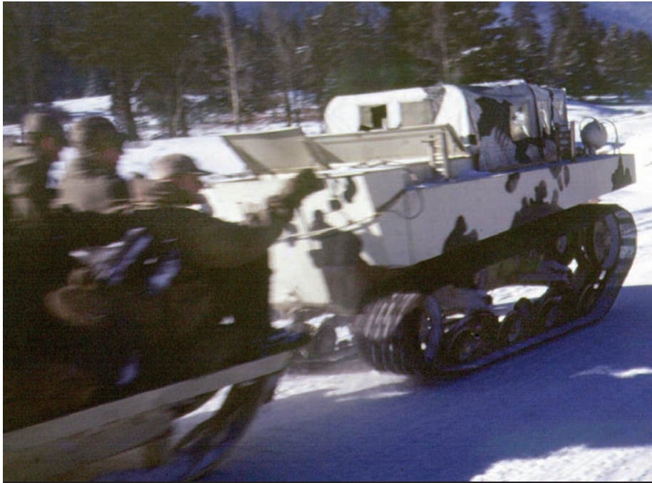
During exercises at Camp Hale, Colorado, in 1943, a camouflaged M-28 cargo carrier speeds along on a snowy landscape while pulling a sled loaded with soldiers of the 10th Mountain Division.
