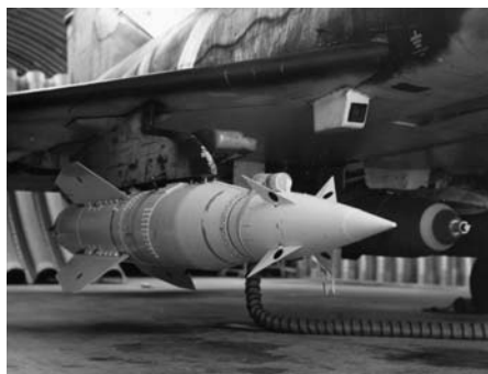
ABOVE: U.S. Air Force F-105 Thunderchiefs refuel over South Vietnam, April 1968. Thunderchiefs had led the first attack against Thanh Hoa Bridge three years earlier. LEFT: An AGM-12C Bullpup air-to-ground missile mounted beneath an Air Force F-4 in Vietnam. The missile was largely ineffective against "the Dragon's Jaw."
