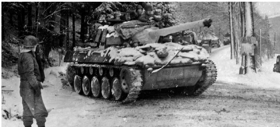
ABOVE: One of the major drawbacks of the open-turret M18 was that its 76 mm gun was little better than the 3-inch gun of the M10. Moreover, many tank destroyer crews preferred the configuration of the M10's fighting compartment. BELOW: M18 Hellcat crews, such as this one the Ardennes in December 1944, reported that their vehicles could go hundreds of miles under trying conditions without requiring major repairs to the armaments or the engine.
