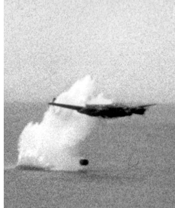
ABOVE: A geyser of water obscures the distinctive twin tail of a modified Lancaster bomber during a training run as it drops a dummy version of the water-skipping Upkeep bomb developed for the top secret raid on Germany's hydroelectric dams in May 1943. ABOVE, LEFT: At the Reculver bombing range in Kent, a modified Lancaster bomber releases its dummy Upkeep during training in the spring of 1943. ABOVE, RIGHT: This still shot taken from a movie shows Barnes Wallis and others watching a practice bomb strike the shoreline during a training flight by members of RAF 617 Squadron at Reculver bombing range, Kent. Wallis is the inventor of Upkeep, the "bouncing bomb" designed to skip across water to destroy hydroelectric dams in Germany. BELOW, LEFT: Photographed shortly before takeoff on May 16, 1943, for the raid on the Möhne Dam, this closeup of Wing Commander Guy Gibson's modified Lancaster bomber shows the 7,500-lb. "Upkeep," whose shape and size required it to hang partially out of the bomb bay.
