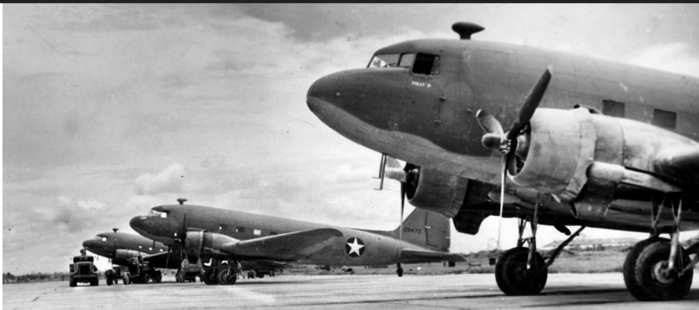
ABOVE: Douglas DC-3 ships standing on the runway at Sookerating Air Base in India. Every ship has a schedule which keeps it in the air the maximum number of hours. The planes that fly over the “Hump” are unloaded a few minutes after landing and take off again for another trip. If possible, each plane must make three trips over the “Hump” each day. OPPOSITE: The remains of a Consolidated C-87 which crashed in the vicinity of Kunming, China. All crewmen were killed in the crash.
