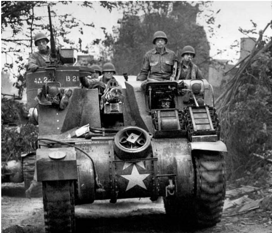
An M7 Priest with the 4th Armored Division moves through Normandy soon after the Division arrived in France in July 1944. The armored, self-propelled 105mm howitzer was first used in battle in October 1942 by British troops in North Africa who thought its rounded .50-caliber machine-gun compartment resembled a priest's pulpit.
