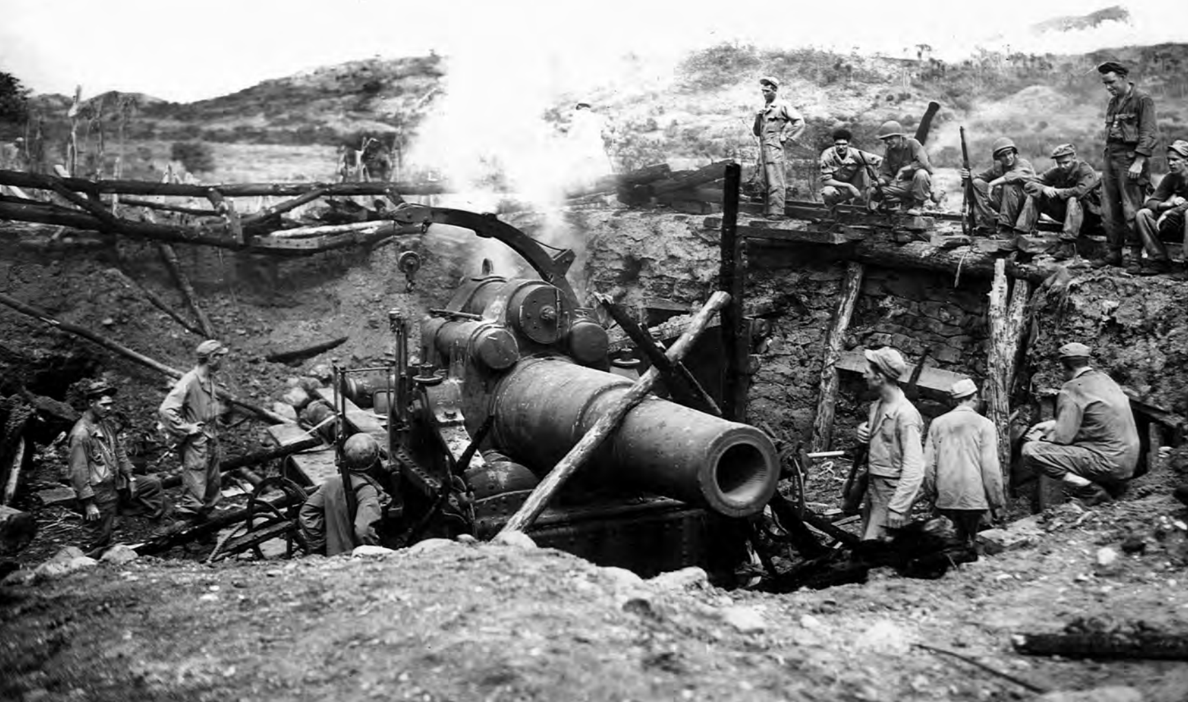
One of two large Japanese guns overlooking the Damortis-Rosario road north of Cataguintangan on Luzon, in an area known as “Two Gun Valley.” This Type 7 30 cm howitzer, with a bore diameter of 12 inches, could fire a 1,300-pound shell more than 9 miles. On February 1, Lt. Erving Peterson’s G Company silenced the mammoth piece with the help of 81 mm mortars. The next day, 1st Battalion followed tanks in to take the second Type 7 gun.
