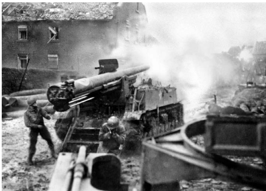
ABOVE: American urban combat teams used the 155mm M12 Motor Carriage "Door Knocker" (pictured here) or a towed 155mm howitzer "Long Tom" for heavy direct fire against fortified German positions at Aachen. TOP: Tech Sergeant Chester Szczekocki uses a flamethrower in Chemical Warfare training, June 27 1944, in Louisiana. The Americans used flamethrowers to subdue diehard German defenders in Aachen. OPPOSITE: With troops of the 36th Armored Infantry Regiment along for a ride, an M4 Sherman medium tank of the U.S. 3rd Armored Division rolls through the Stolberg on October 14, 1944. The fight for Aachen and the surrounding area was arduous, a taste of things to come as Allied troops struck deeper into Nazi Germany.
